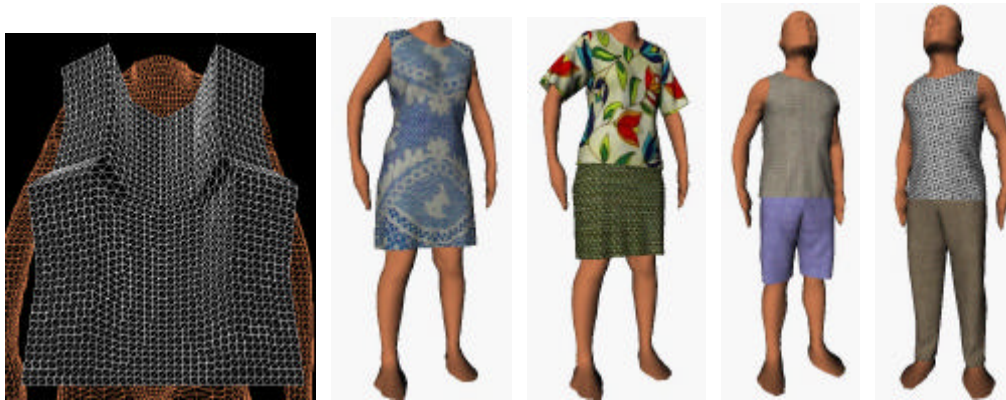
Figure 8: Pattern pieces for a shirt with a rectangular topology mesh, and examples of body scans with clothing fitted on them. Textures have been mapped onto the patterns to enhance realism.
